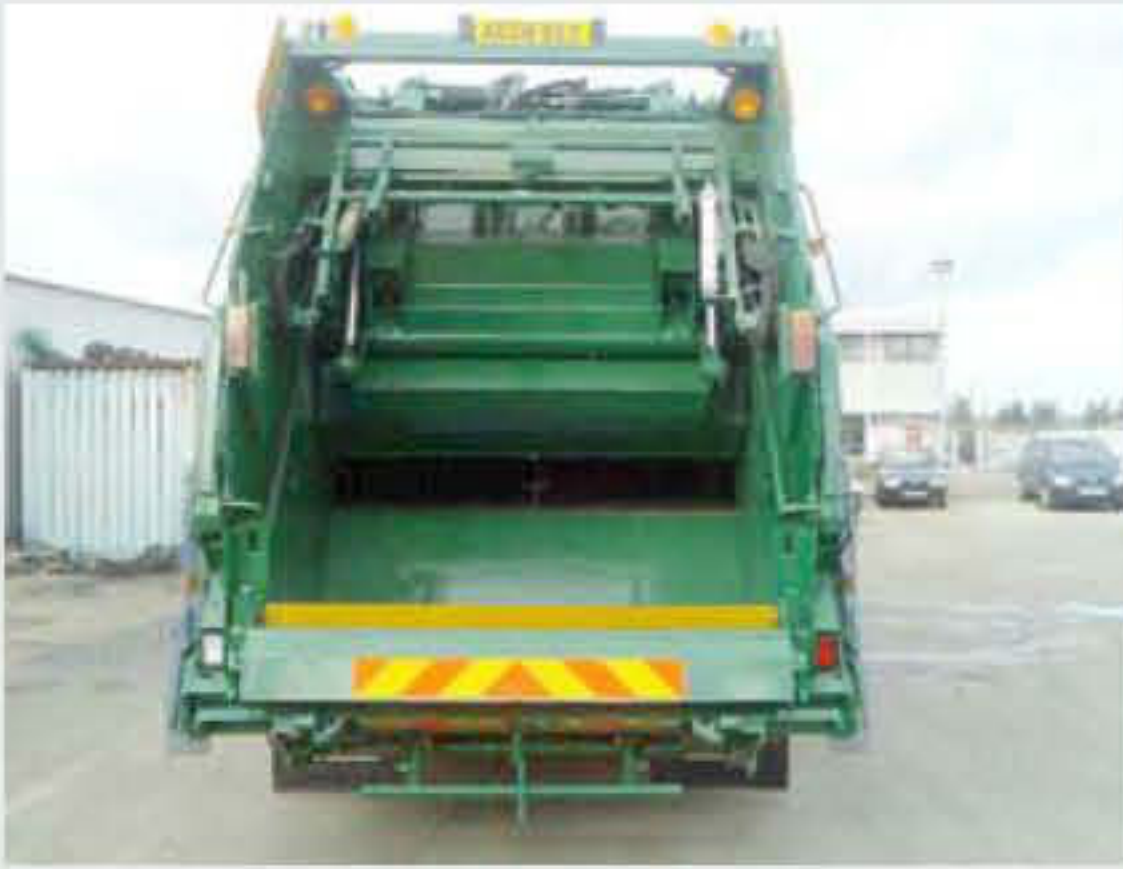
Low loading height and large loading width are maintained for loading bags or bulky waste.
