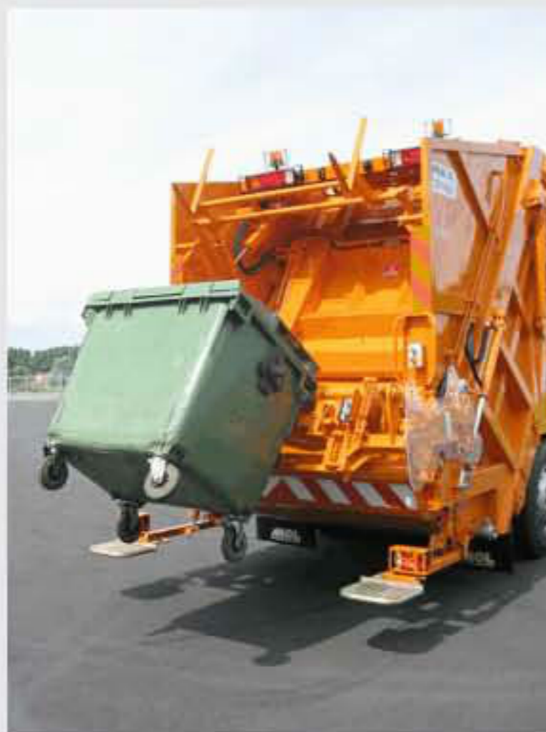
Lifting with comb or with arms: 4-wheeled bins according to DIN EN 840-2.
