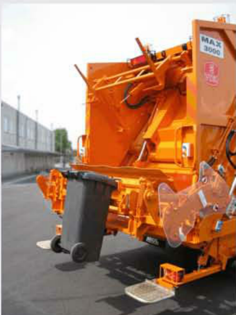
Lifting with comb: 2-wheeled bins according to DIN EN 840-1.
