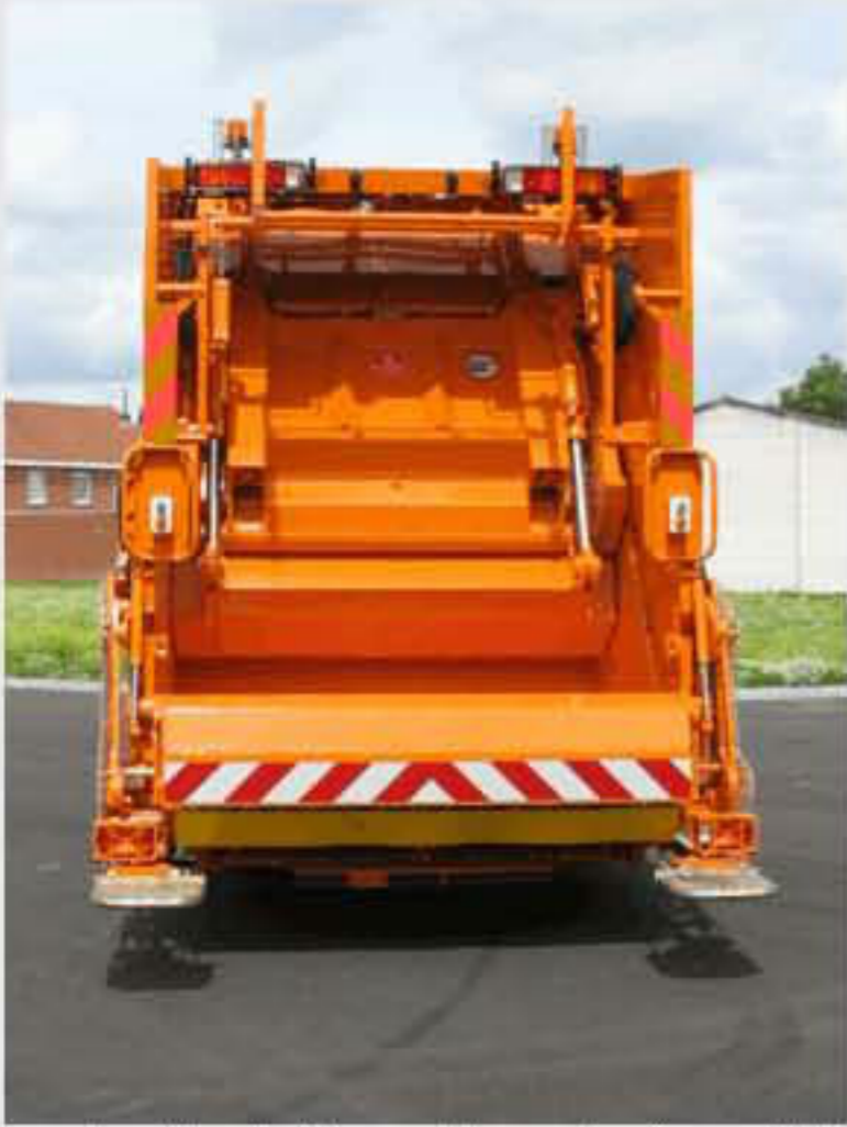
Low loading height and large loading width are maintained allowing for bags and bulky waste to be loaded.
