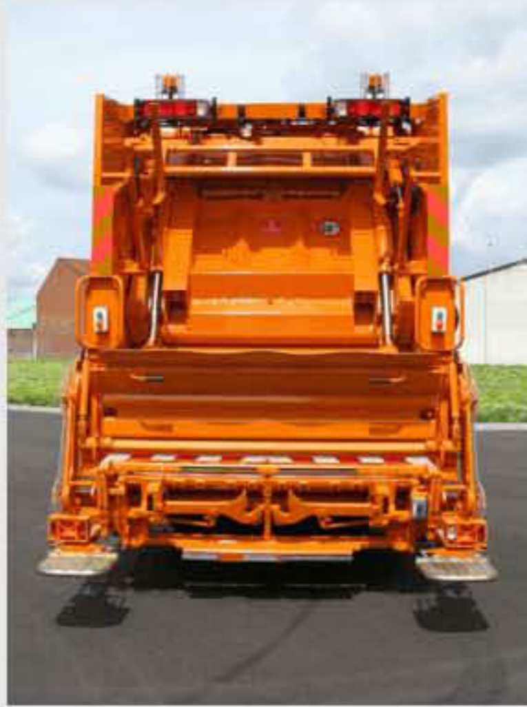
The up and down movement of the hopper flap is electro-hydraulically operated. Continuous working of compacting system with raised hopper flap.
