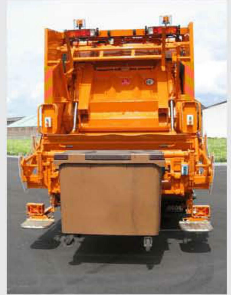
The lid opener and container support are electro-pneumatically operated.
