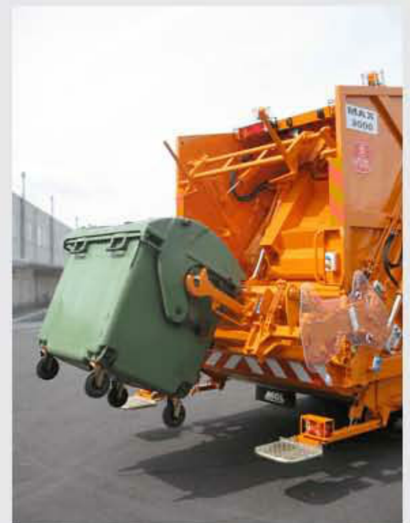
Lifting with comb or with arms: 4-wheeled bins according to DIN EN 840-3.
